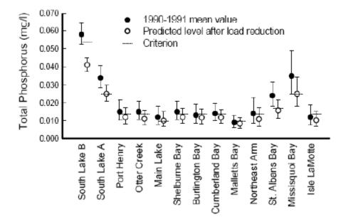
Predicted phosphorus concentrations in Lake Champlain segments following targeted load reductions, compared with 1991 measured mean levels and in-lake criteria values (from Table 2). Error bars show 95% confidence intervals for the existing mean and predicted phosphorus concentrations. The predicted concentrations and criteria values are listed below. (Figure modified from Vermont DEC and New York State DEC 1997.)
