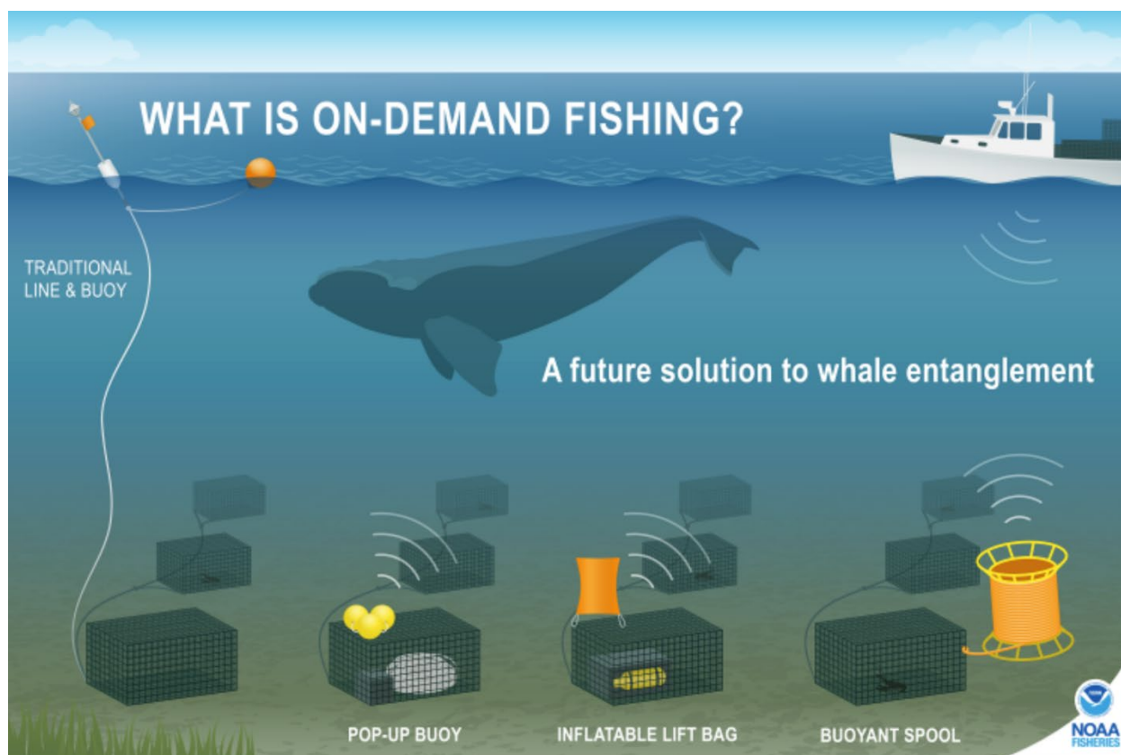
Figure 1: Three Types of On-Demand Systems. (NOAA Fisheries)
